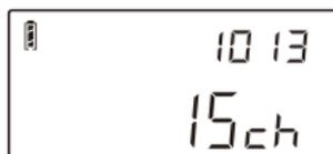
when entering the LW/MW ETM memory. In this example, "1013" indicates that the current listening time is between 10:00 and 13:59, whereas "15ch" indicates that the last time an ETM+ scan was done during this time-range the device found 15 broadcasting frequencies.
