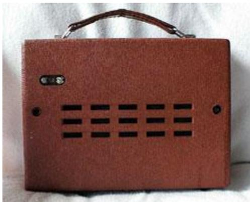
The plastic part of the case is ABS, and appears very sturdy. Although the radio I have shows obvious signs of abuse, there are no cracks or chips anywhere on the case. The P780 was manufactured in this reddish-brown called "Ginger". The case is pebbly to resist fingerprints (a technique adopted almost universally by other manufacturers a decade after this radio appeared). No phone or external power jacks, but a pair of terminals for connecting a long wire antenna.
