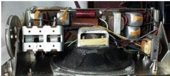
A view looking at the radio from the bottom. Notice the large (and taped!) IF transformers and capacitors.
